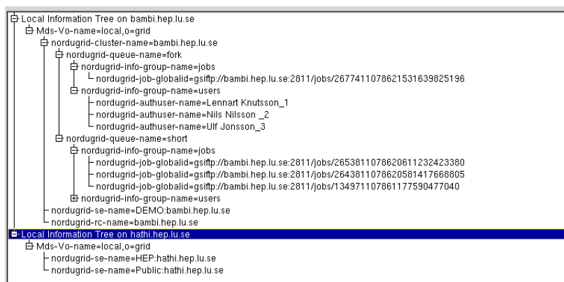
Figure 2: The local information tree on two resources. The first machine bambi.hep.lu.se provides both computing, storage and data indexing services while the second resource hathi.hep.lu.se hosts two storage elements.
