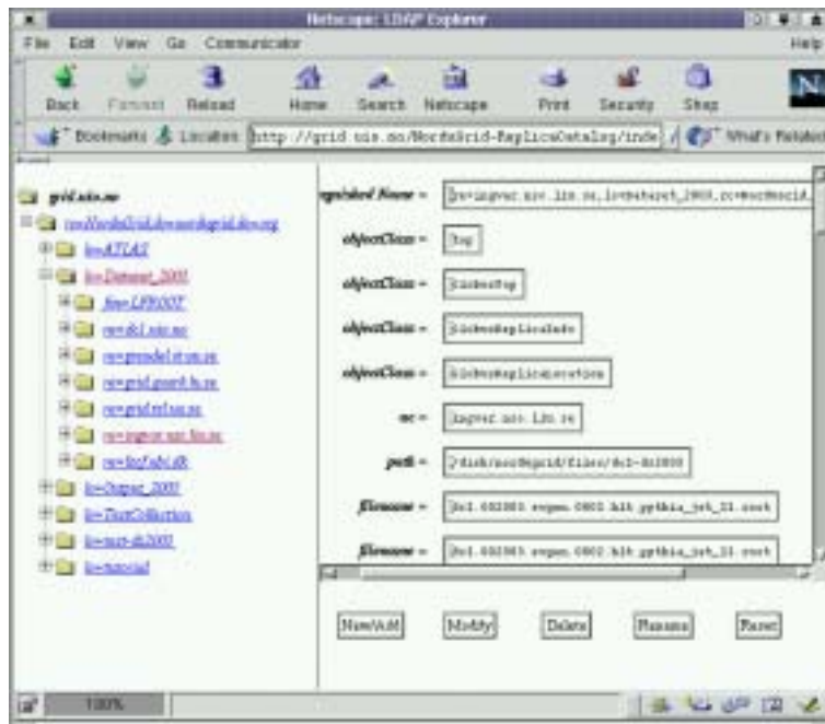
Figure 5: A snapshot of the Replica Browser showing the dataset 2003 input-files as registered in the Replica Catalog.
